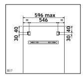
Fix the brackets according to the measurements shown in the figure, by using four 3.5 x 16 screws.
